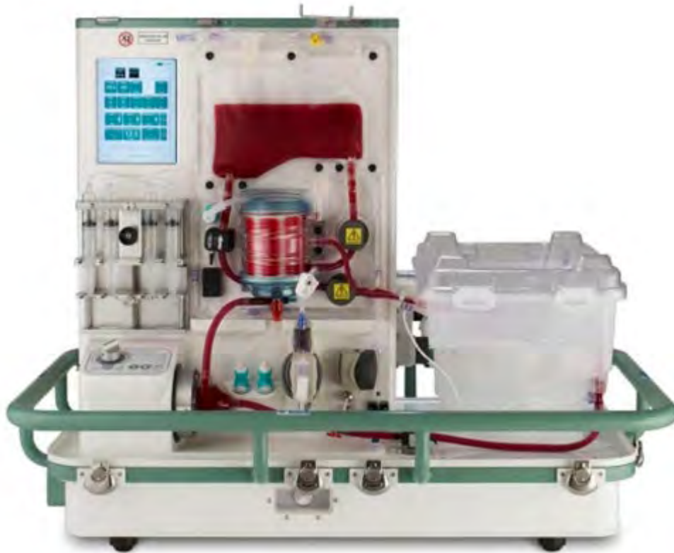
NMP device and circuit. OrganOx metra (generation 1)
